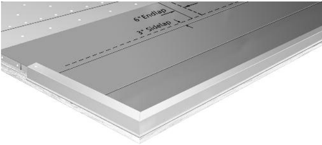
Figure 5-18: Apply roof edge metal.
